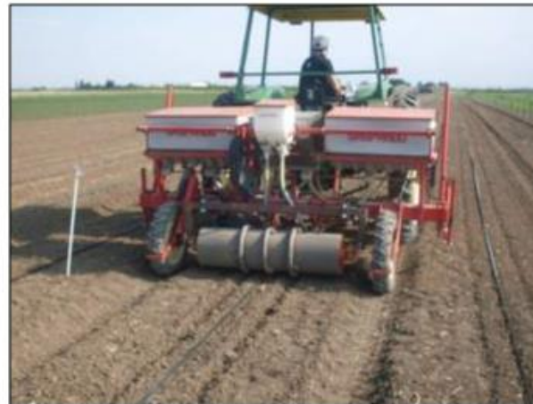
Tomato trials in the south of Italy were applied using Gaspardo microgranule applicator before transplanting. Twin-rows plantation. •Product was applied in furrow under the plantation line.
